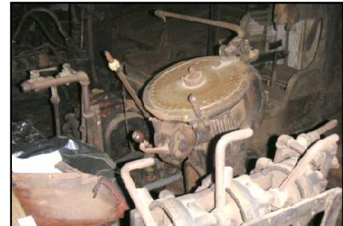
Set Works dial shown with Setters seat in bottom left corner.
